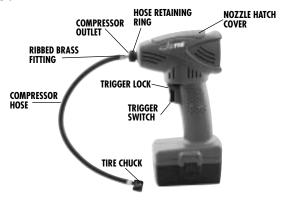
The Compressor On/Off Switch controls operation of the compressor. It conveniently is depressed and released to control inflation. An exact pressure is obtained by observing the gauge and releasing the trigger when the correct pressure is achieved. For longer inflation operations, the Trigger Lock can be moved laterally to lock the trigger in the ON position. Pushing the trigger lock to the opposite direction releases the trigger (OFF) and inflation stops.
